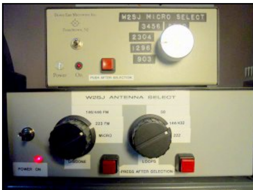
Home brew switching box consisting of (4) SP4T SMA latching relays to route the antennas to the proper transceiver or transverter.
